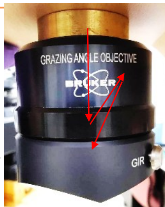
Fig 1: View (left) and measurement (right) modes in the Bruker grazing angle objective.
